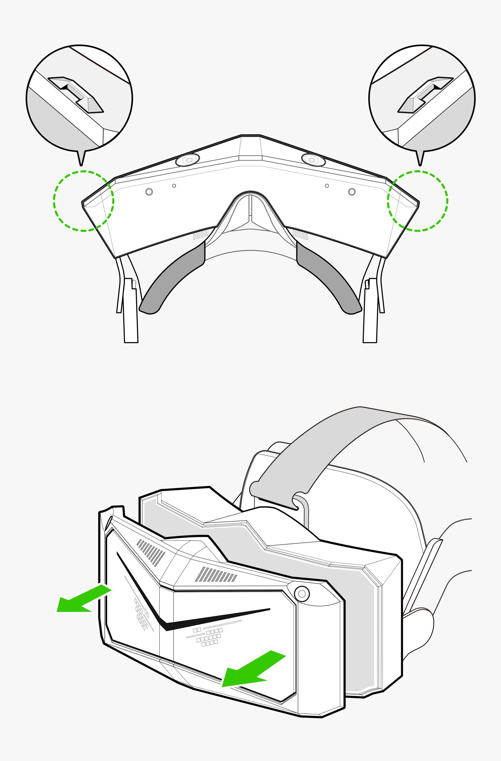
Step 2: Install and fasten the another Cover to be replaced according to the interface.
